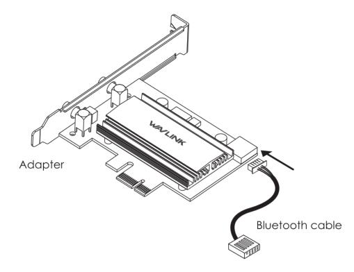
3. Find the corresponding PCI-E slot, then insert the adapter carefully.
