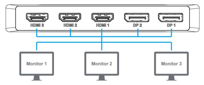
(Max. Three simultaneous video outputs are supported, single/dual/triple 4K@60Hz)
