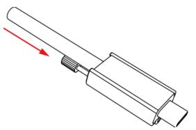
2. Align the bolt with the fixing hole, then please connect it to the upstream Thunderbolt™ 4 port.
