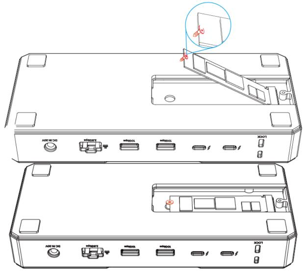
4. Peel off the protective films on both sides of thermal silicone pad and stick it to SSD.
