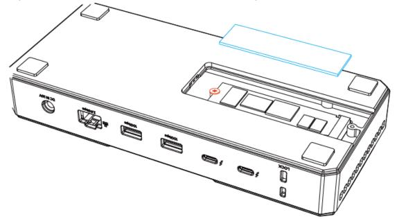
5. Reassemble the cover after aligning the contacts, then screw the screws on the back cover.
