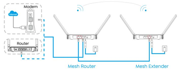
2. After mesh router is paired with mesh extender section, then connect the **WAN** port of the extender to **LAN** port of your router.
